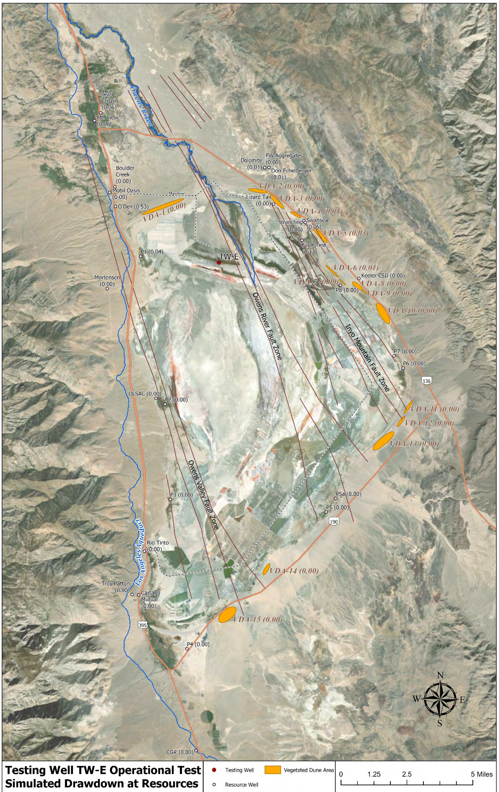
Figure 14: Simulated Shallow Aquifer Drawdown (ft) at Groundwater-Dependent Resources due to Operational Test of TW-E
