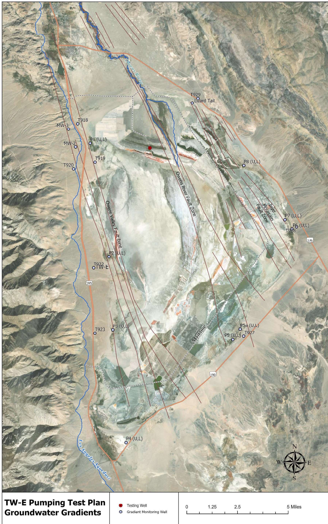
Figure 6: Monitoring Well Locations Utilized for Groundwater Gradients
