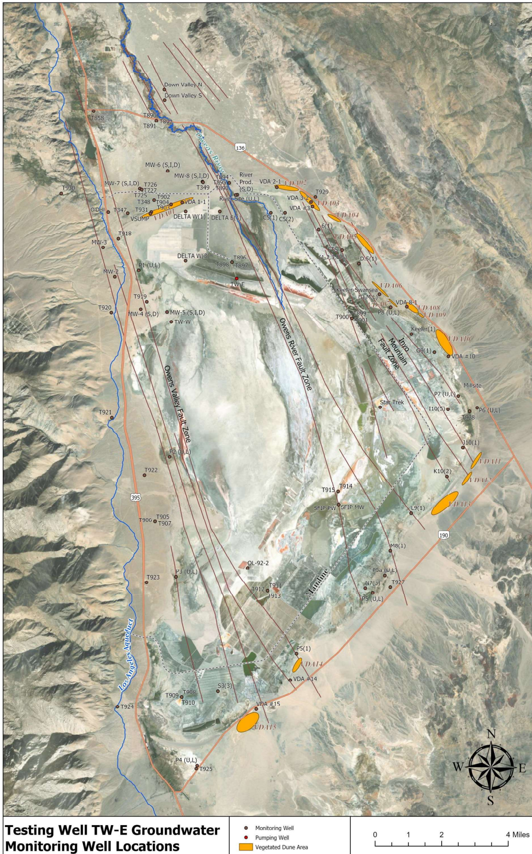
Figure 3: Monitoring Well Locations during the Pumping Test of TW-E
