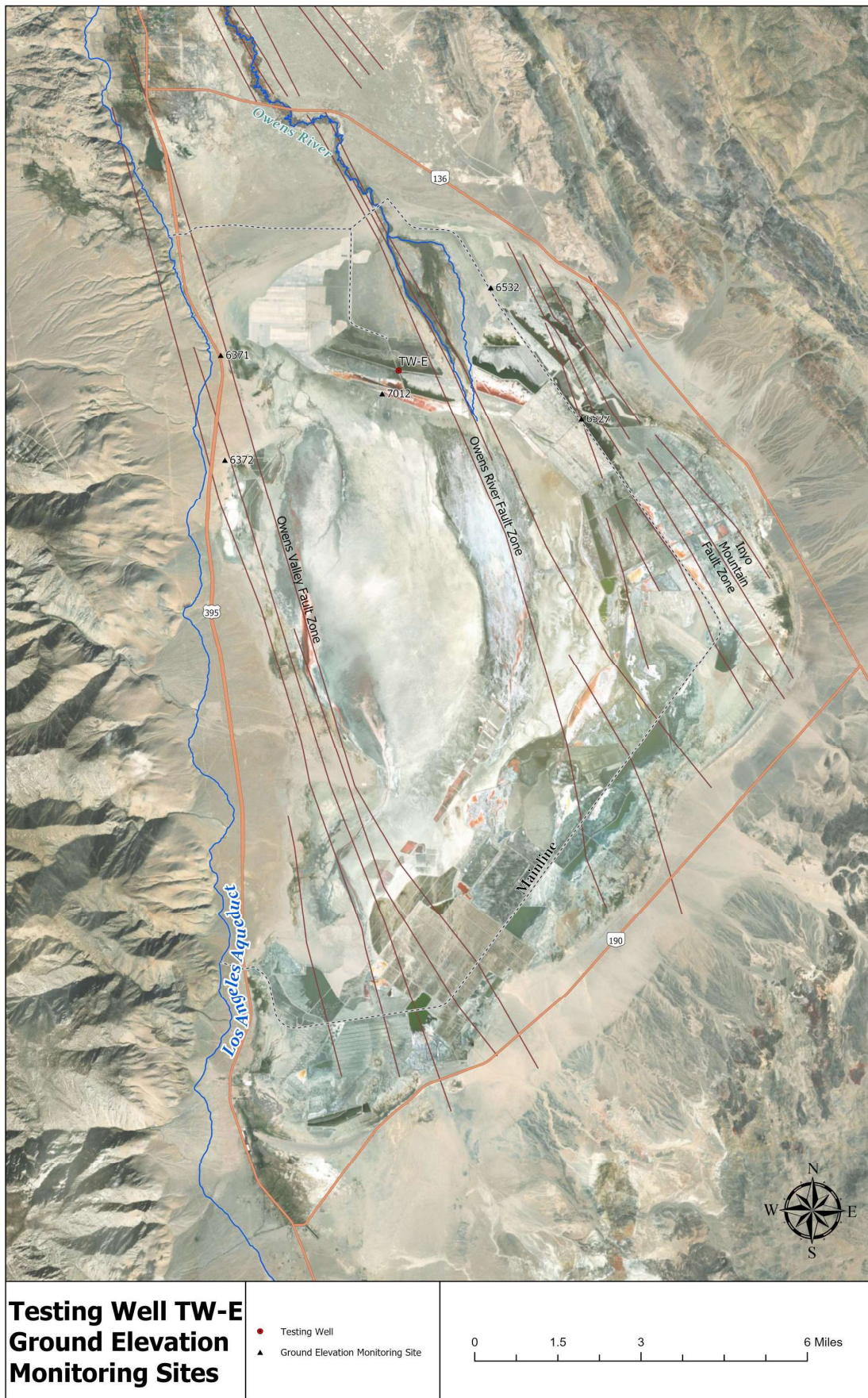
Figure 7: Ground Elevation Monitoring Sites during Pumping Test of TW-E
