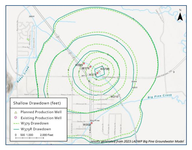
FIGURE 8 - SHALLOW AQUIFER GROUNDWATER DRAWDOWN (FT) FROM OPERATING EXISTING W379 AND REPLACEMENT W379R AT 4.3 CFS FOR ONE YEAR
