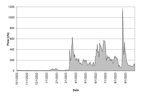
Figure 2-2. Langemann and Weir Release to Delta.
