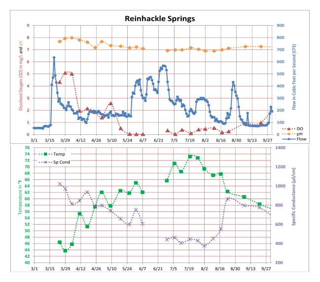
Figure 3-5. 2023 LOR Reinhackle Springs. LOR Flow with DO, pH, Temp, and Sp Cond at Reinhackle Springs. Gaps in water quality parameters indicate measurements missed due to site inaccessibility.
