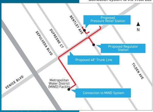
Project Schedule Summer 2018 – Summer 2020 Region West Los Angeles Angeles area. The project will provide an emergency connection to the Metropolitan Water District of Southern California (MWD) water supply by constructing a new trunk line that will be connected to an existing pipeline. The new steel trunk line will be between 20-inches and 54-inches in diameter and extend approximately 1,700 feet under Sepulveda Blvd. and Venice Blvd. within the City of Los Angeles and Culver City.
