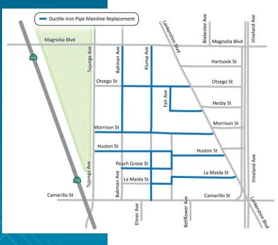
Project Schedule December 2019 – March 2021 **Region** North Hollywood and Klump Avenue. The existing pipes were installed between 1925 and 1927 and are near the end of their service life. The new pipe is 6-inch ductile iron pipe that is more durable and resilient than the cast-iron pipe currently in place. The project is part of LADWP's overall plan to replace aging water infrastructure.
