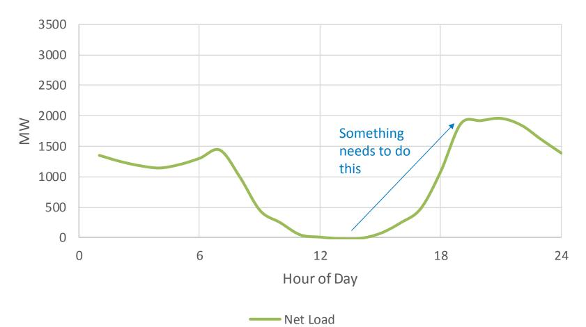
This presents some problems as we transition from a hydro/thermal based system to an all RE based system. Meeting this net load curve would require turning off all of LADWP's power plants for an hour, then turning them back on, and quickly ramping them back up. This isn't really possible, so we probably couldn't accommodate all this RE generation.
