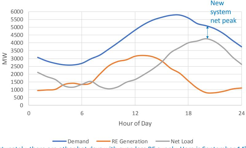
Unfortunately, there are other hot days with even less RE supply. Here is September 14<sup>th</sup>. We have less wind, slightly earlier sunset, and a slightly later peak. Our 5,000 MW of wind and solar capacity is producing less than 500 MW and our net peak demand is over 4,000 MW. Even with Castaic, we need about 3,000 MW of additional capacity.
