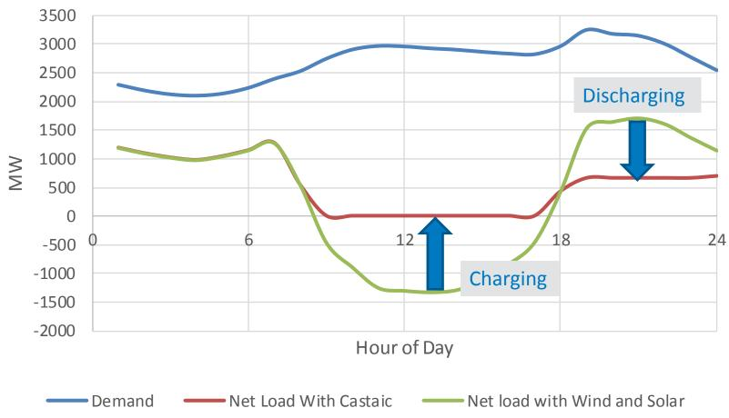
Adding in Castaic eliminates curtailment on Feb 20. But we have just about saturated the power capacity of this storage plant. More solar on this day will create more overgeneration.
