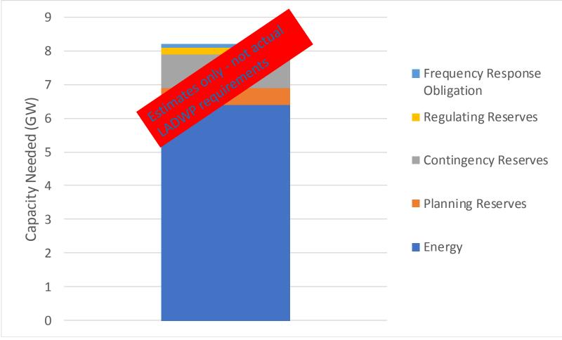
And LADWP also needs to plan around outages of their transmission network and generation resources. This means even more "firm" capacity is needed during the hours of peak demand. This capacity is unlikely to be provided from wind and solar, because as we have shown, there is relatively little solar and wind available during the hours of peak demand.
