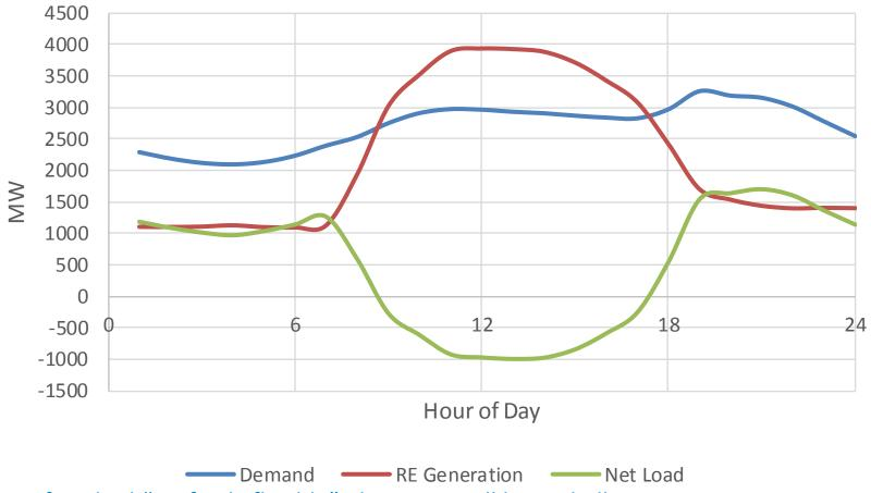
Even if we had "perfectly flexible" plants, we still have challenges as we increase RE penetration. Here is a case where we try to get 60% of LADWP's energy from RE (including 1,800 MW of wind and 2,700 MW of solar). On this day the supply of RE exceeds demand.
