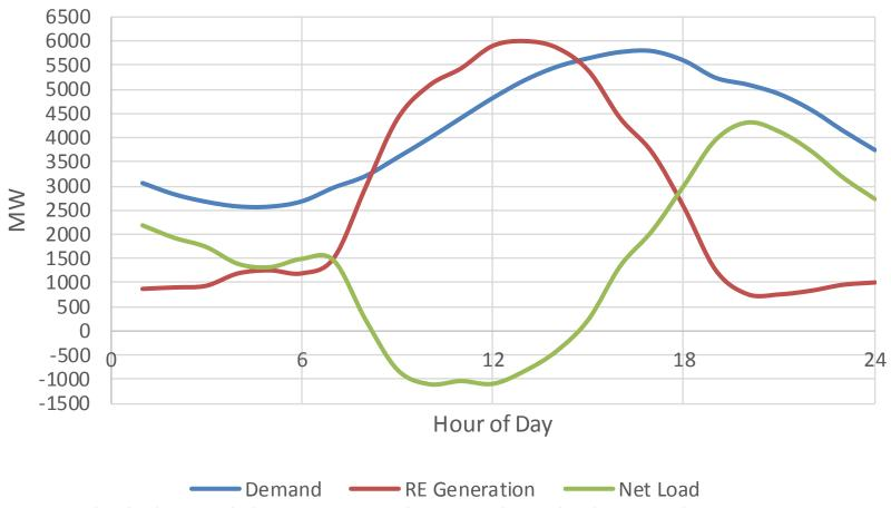
Here is a very high demand day in a case where we have built enough RE to meet 100% of demand. Our net load peaks at about 4,300 MW. So our storage case (Castaic plus 3 GW of batteries) could provide us almost enough capacity to meet the energy requirements. This ignores reserve requirements, so we do NOT have a reliable system.
