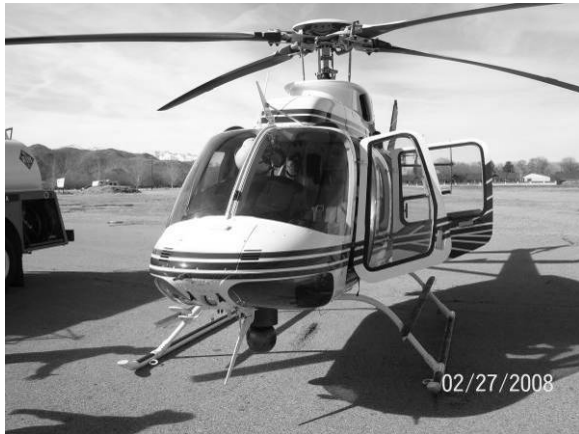
Seasonal Habitat Flow Figure 2. LADWP Helicopter with Mounted FLIR Unit
