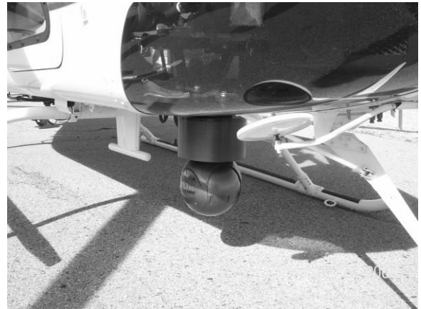
Seasonal Habitat Flow Figure 2. LADWP Helicopter with Mounted FLIR Unit
