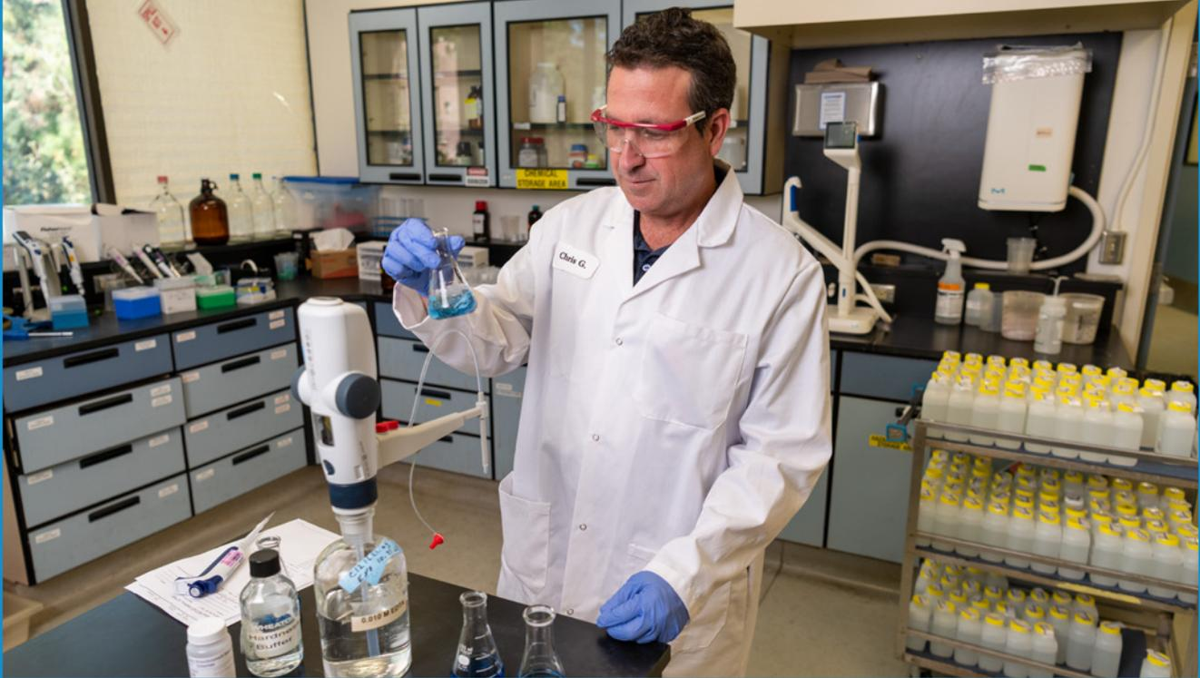
One of LADWP's chemists works on determining total hardness in drinking water using a method known as SM2340C (EDTA Titration), which is one of the 220,000 test parameters LADWP utilizes in order to ensure safe drinking water.
