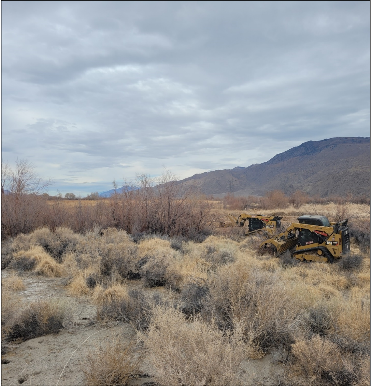
Tamarisk Figure 5. Turbosaw at Lower Goose Lake used to cut tamarisk trees and grapple rake for collecting and consolidation of tamarisk slash.
