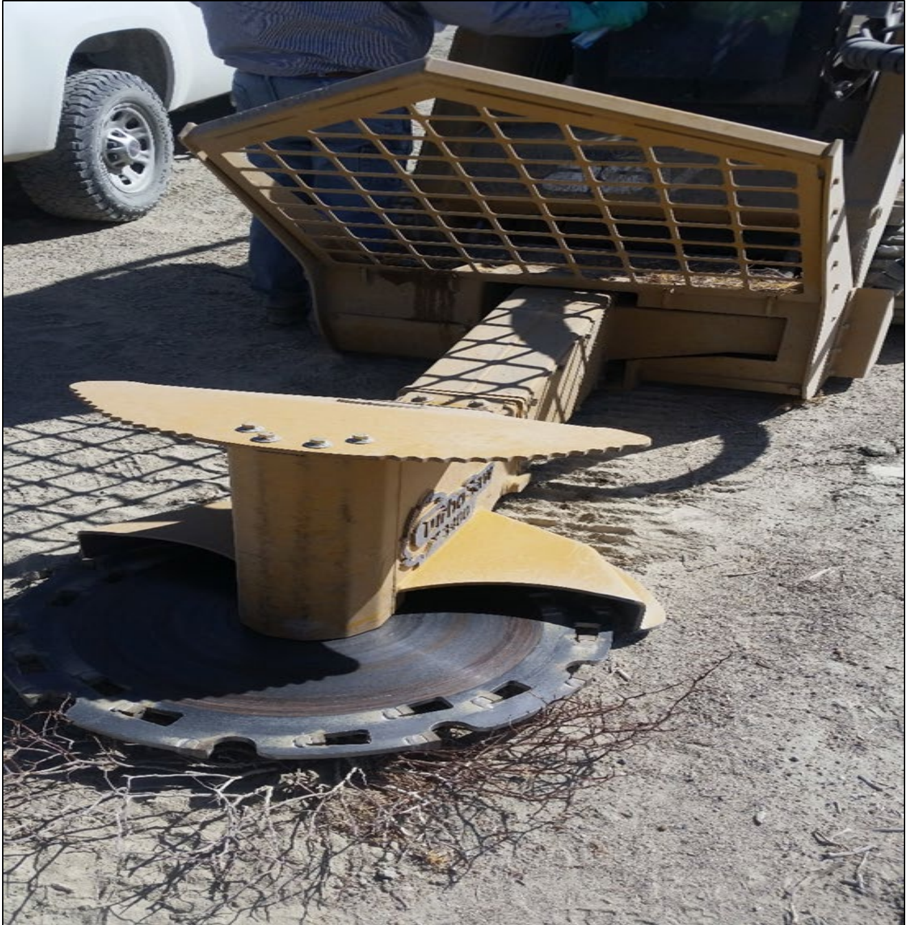
Saltcedar Figure 2. Turbosaw attachment used to cut larger diameter tamarisk trees and apply herbicide to the cut stumps
